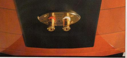
A single set of binding posts means bi-wiring is not an option, but proprietary internal wiring of silver feeds all drivers extends both bandwidth and improves sonic clarity while maintaining the desirable energy-termination characteristics of polypropylene co-polymer.
