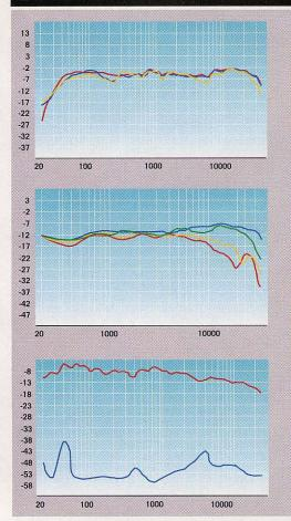
The lab measurements revealed a superbly uniform mid/treble, devoid of usual cabinet edge diffraction anomalies. The aurally dominant central region, at least 400Hz to 4kHz, met unprecedentedly narrow ±0.75dB amplitude limits, within the stated tolerance for a precision microphone!
